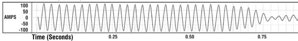
Up to 10 times more power is necessary to start a compressor than to run one. During a hot summer, an air conditioning system can start up more than 4000 times.
